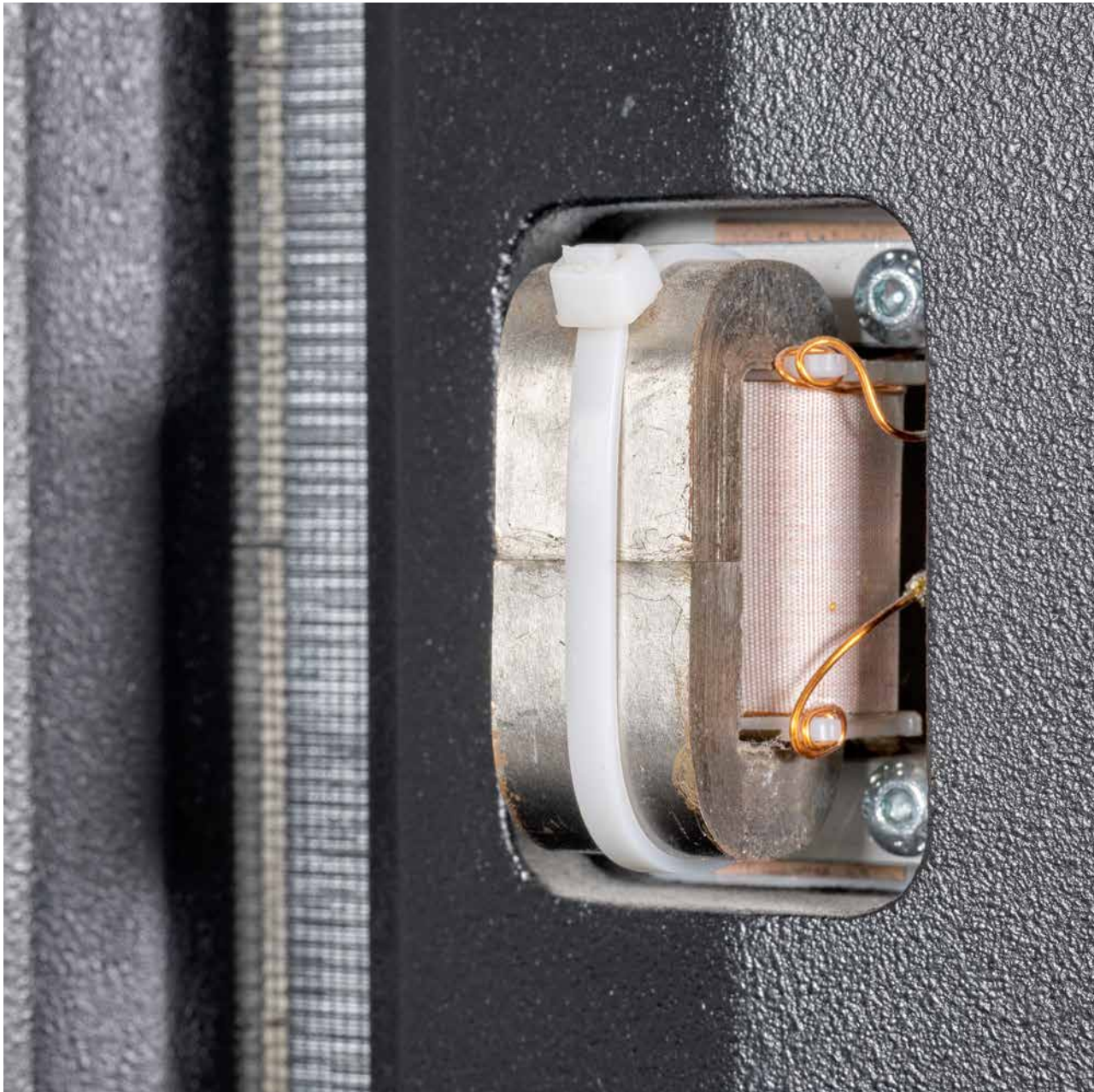
A necessary transformer elevates the impedance of the razor-thin ribbon to an amplifier-friendly level; openly exposed, it's secured to the back wall of the BB-15's housing.
