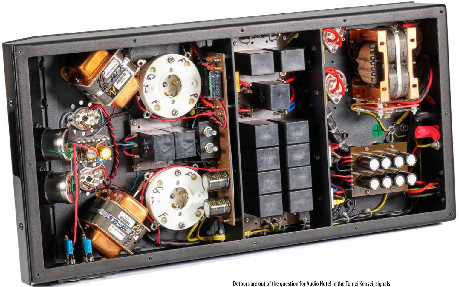
Detours are out of the question for Audio Note! In the Tomei Kensei, signals undergo amplification via the shortest possible paths. The trade-off for this specificity is that the input must have an unusual position: on the front left-hand side of the housing. This is the blue component in the bottom left of the image.
